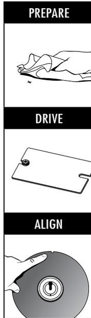
1. Mark location where PowerGrip is to be installed. Prepare membrane surface at each location following roof system manufacturer's requirements.
