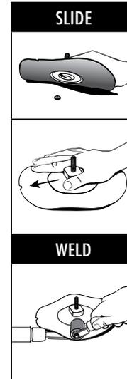
4. Slide the assembly over the head of the fastener to position the PowerGrip in the proper location.
