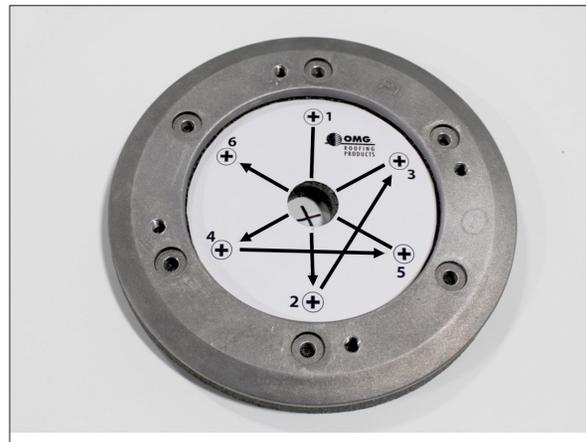
**STEP 4:** Once the base plate is attached to the roof, loose lay the cover plate over the base plate by aligning the bolt holes. Once the bolt holes are properly aligned, mark the cover plate and membrane as shown to help re-align the cover plate for final installation in step 6.
