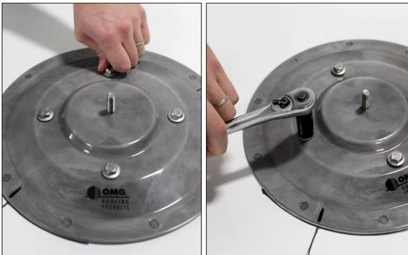
**STEP 8:** Once the cover plate is secured to the base plate, inspect to ensure that water block sealant has squeezed out around the edges of the top disc. Apply more water block around the edge of the disc if necessary.
