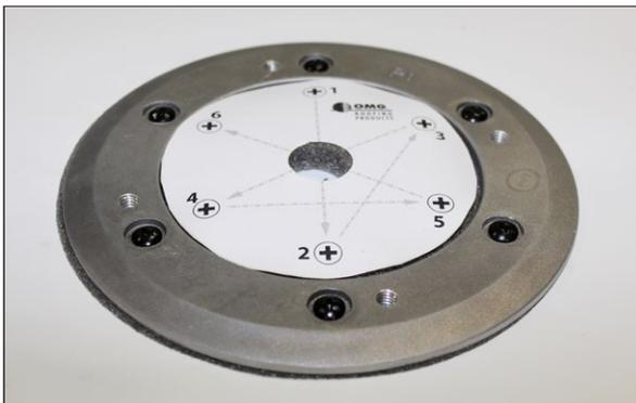
**STEP 3:** Mechanically attach the base plate through the membrane and into the roof deck using appropriate OMG Roofing Fasteners (sold separately). Add ½-in. to the length of the fastener to compensate for the base plate thickness. Special care should be given to drive the fasteners perpendicular to the deck, not at an angle. Do not over or under drive fasteners.
