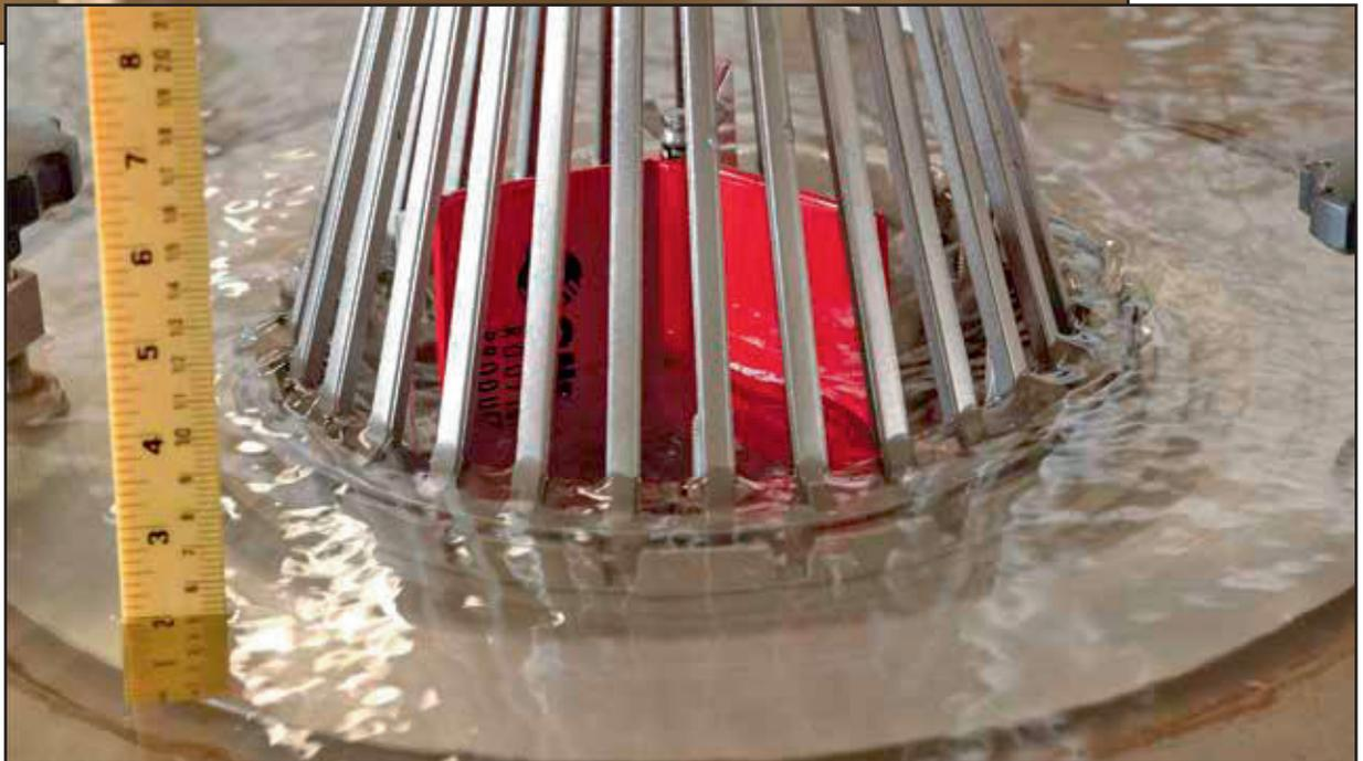
Figure 6 – A patented roof drain featuring a vortex breaker within a drain flow test rig breaks the vortex and flows to the maximum capacity of the storm drain piping while maintaining a consistent head of water. A video of the test can be seen at [www.omgroofing.com/roof-drains-and-vents/RedLine-AFR.html](http://www.omgroofing.com/roof-drains-and-vents/RedLine-AFR.html).
